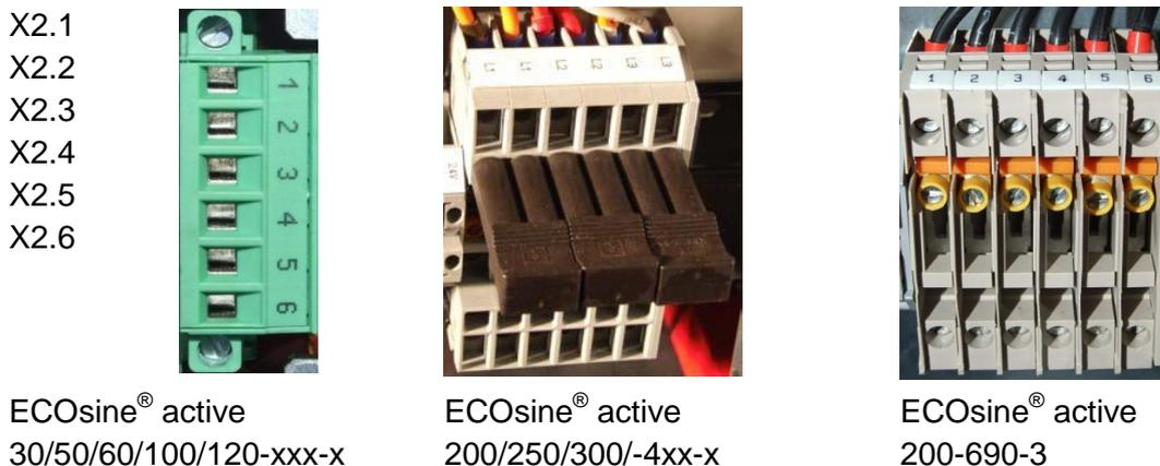
Fig. 54: X2 terminal strip – ext. current transformers
