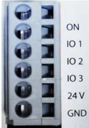
Fig. 63: X5 terminal strip – digital inputs and outputs (ECOsine® active 30/50/60/100/120-xxx-x)
