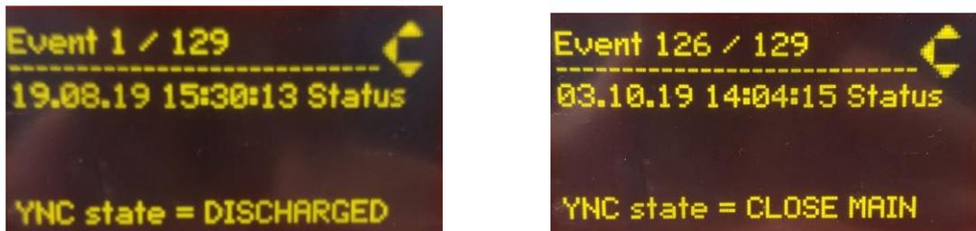
Figure 9-25 Display module screen, events examples
