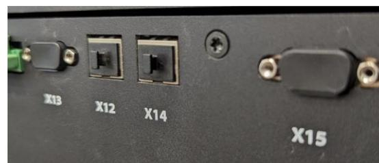
Figure 8-35 Example of communication ports with covers installed.
